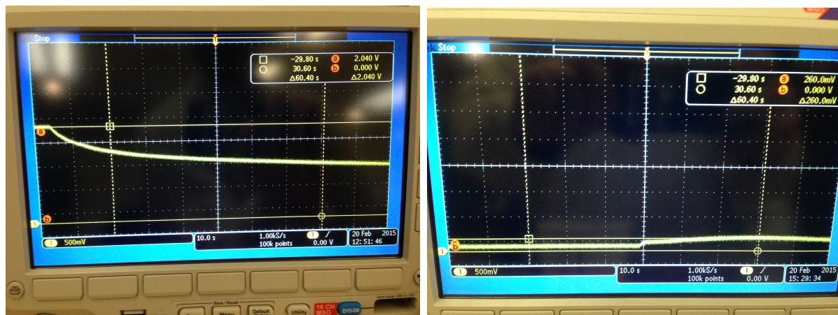
Figure 5.3.1.2. Oscilloscope Voltage Readings When Blood Sugar Was Applied to Test Strip
